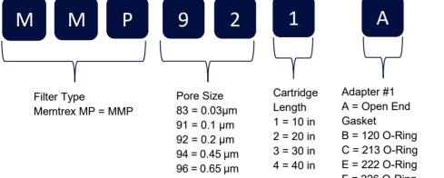
F = 226 O-Ring J = 020 O-Ring Q = 222 O-Ring with stainless steel Insert3 Z =226 O-Ring with stainless steel Insert3
