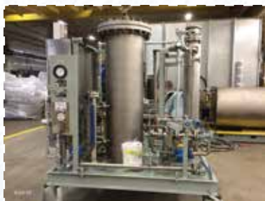
Ex: Stainless and Carbon Steel heated system with Pre-filter. Explosion-Proof with purged electrical enclosure and transmitters. 2014
