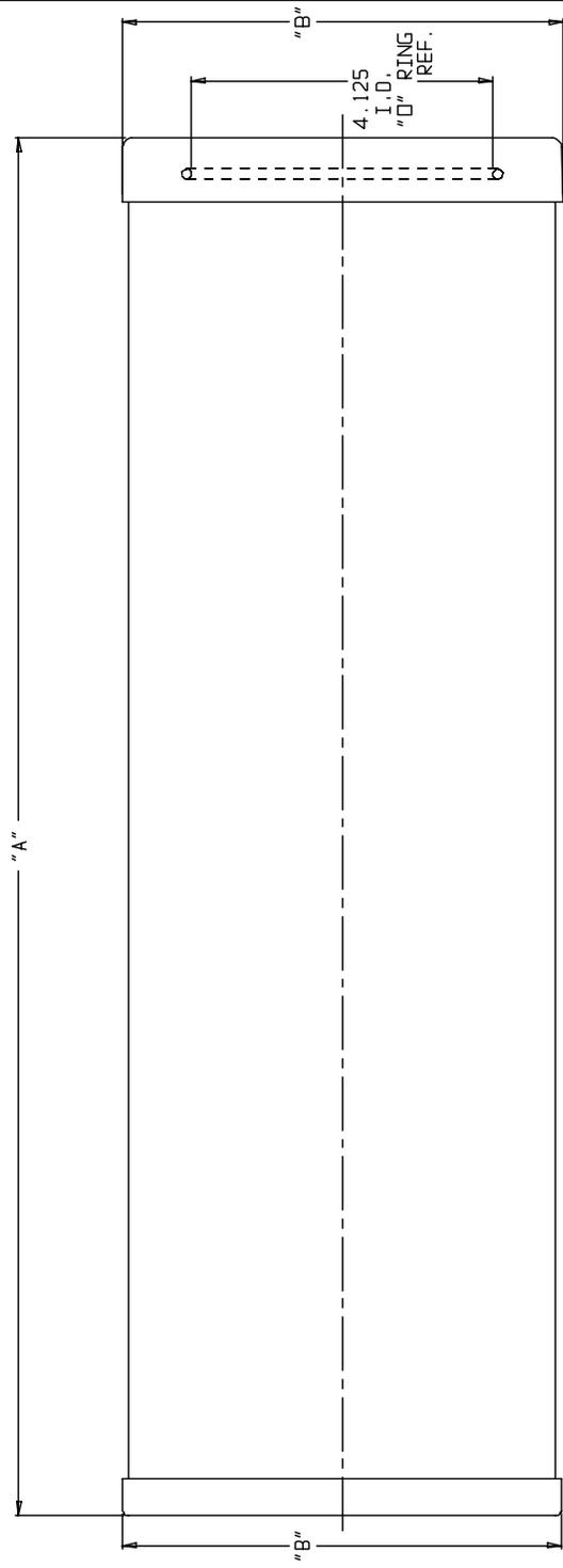
NOTE: USE PARKER SUPER D-LUBE ON "D" RING BEFORE INSTALLING IN VESSEL.
