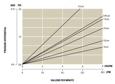
For liquids other than water, multiply the pressure drop by the fluid viscosity in centipoise.
