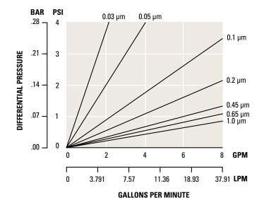
This chart represents typical water flow per 10" cartridge length. The test fluid is water at ambient temperature. Extrapolation for multiple elements tends to be linear, but as flows increase the  $\Delta P$  of the housing becomes more apparent.
