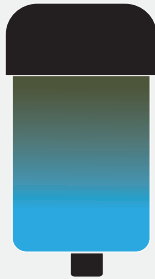
A green/brown color indicates that the silica gel has absorbed oil, but is not exposed to moisture.
